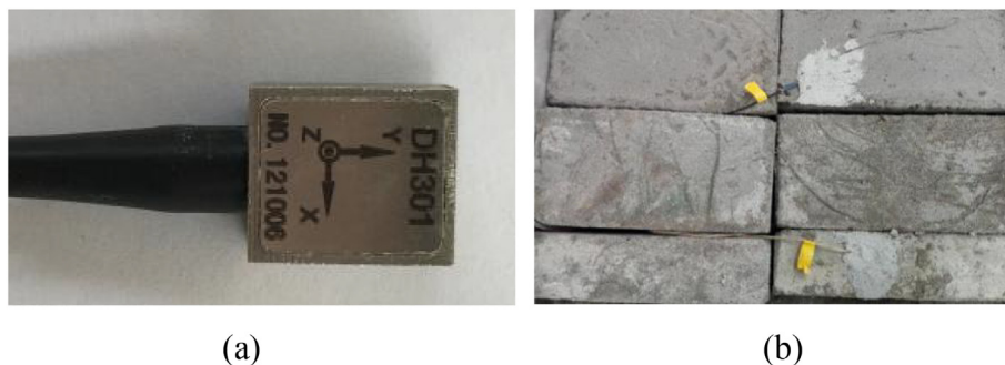
Fig. 8. Acceleration sensor and its placement.
